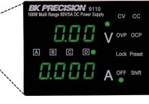
Models 9110 and 9111 are a new type of power supply. Unlike conventional power supplies with fixed output ratings, they automatically recalculate voltage and current limits for each setting, providing any Volt/Amp combination within the rated power. By providing greatly expanded choices of maximum power Volt/Amp combinations, users can cut down on the number of power supplies required and free up valuable bench space.
